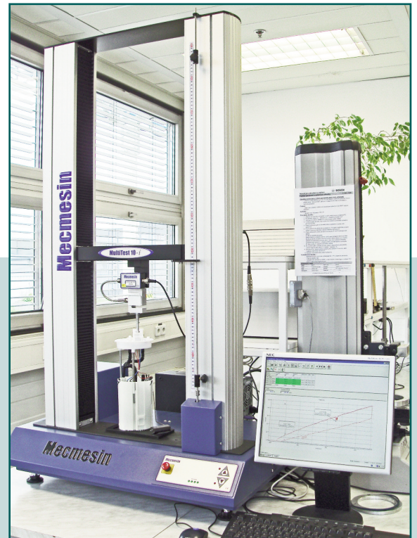
The complete system with a pump assembly under test
