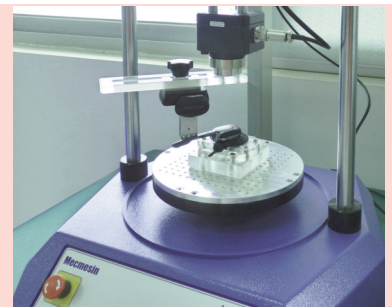
On-ear headset microphone arm test
