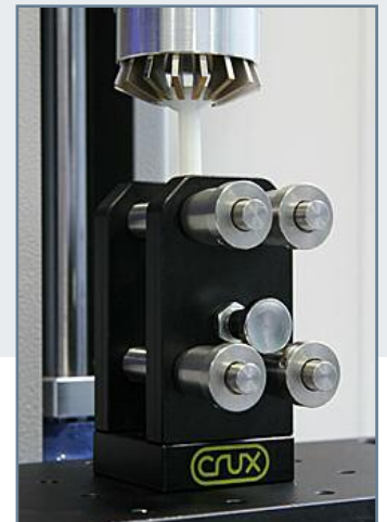
Injector pen training device in upper multi-jaw grip and lower bespoke fixture
