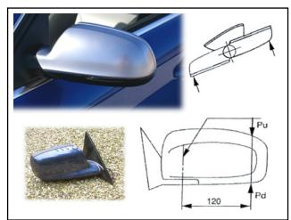
Automotive side mirror durability testing specification
