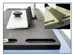
Beltline molding deflection testing, including T-slot locating design
