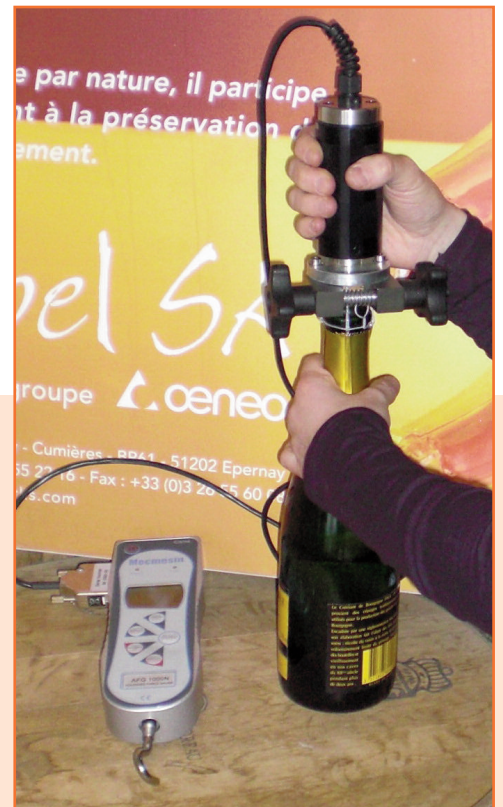
Testing cork extraction force
