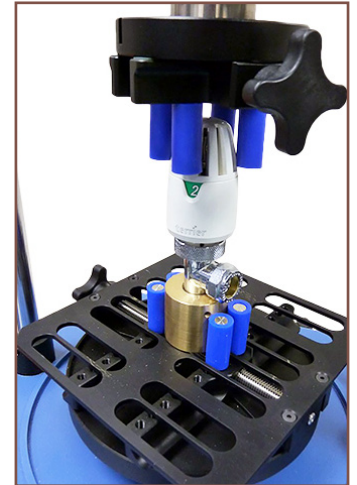
TRV undergoing torque to turn testing on the Vortex
