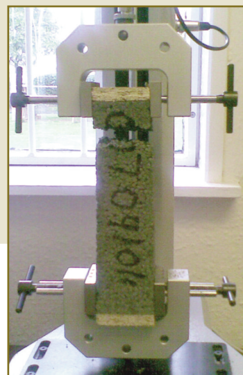
Sample shown has passed test as bond is still in tact
