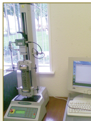
The pre-programmed MultiTest-x enables automatic transfer of data to a PC
