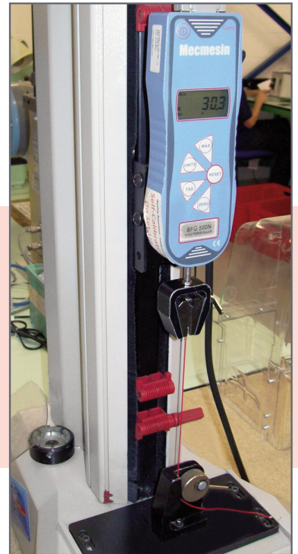
Tensile test on crimp joints of cables
