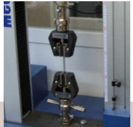
Tensile test on shutter material
