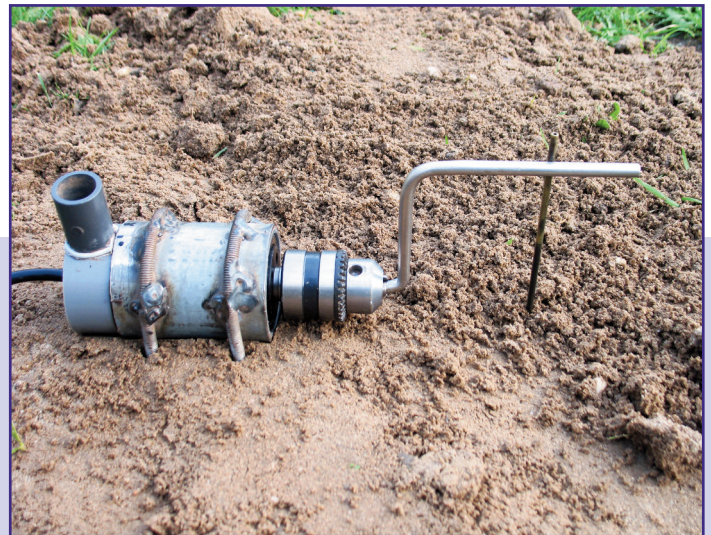
Torque screwdriver in casing in field trial
