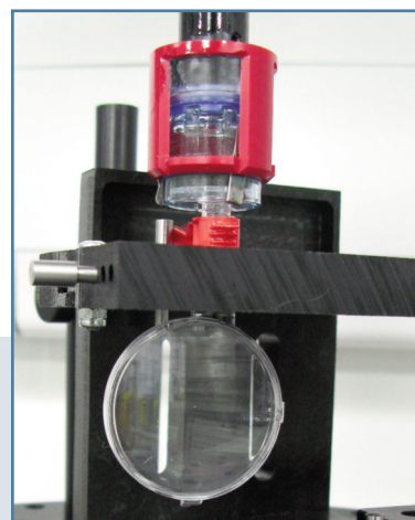
Spectacle dial presented for testing in special test fixture
