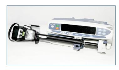
precisely accurate in order to ensure early occlusion detection, and guarantee a consistent dosage reaches the patient. Cardinal Health, therefore, required a tool with which to perform regular calibration of the occlusion-monitoring sensor.
