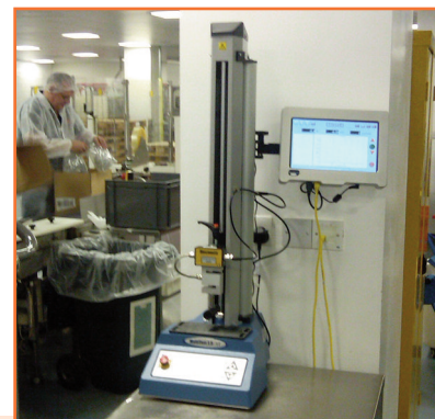
The MultiTest-xt enables in-line quality checks on the production floor
