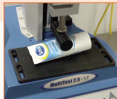
Sample presented for application of compressive force
