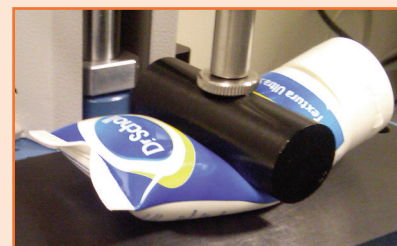
Special compression probe applies force at 60kgf and 100kgf
