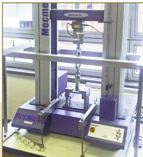
The test stand with custom-made test sample fixtures
