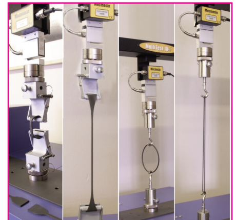
Spring Loaded Fold Grips and Test Hooks used to test different samples
