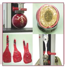
Clockwise from top left: Cricket ball compression test; Ball interior showing cork,wool & leather layers; Leather sample tension test; Leather tension test dumbells (in separated pairs, post test).
